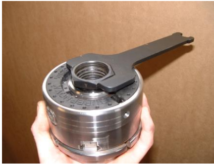
Using 1 1/2” spanner to remover insert from chuck
