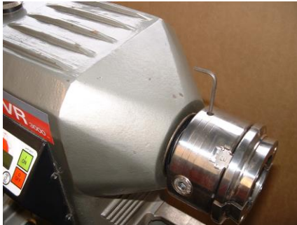
Removing grub screw to release insert
