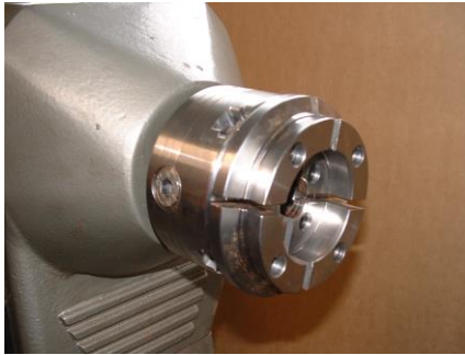
The Supernova 2 chuck on a Nova 3000 DVR lathe
