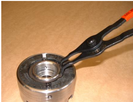
Using Circlip pliers to remove circlip
