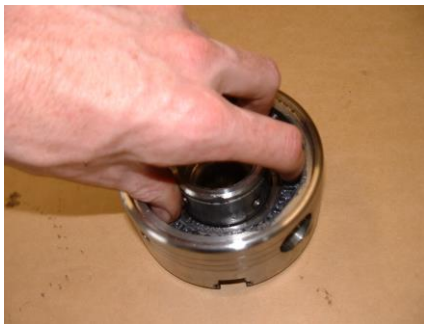
Moving scroll ring back and forth to seat it
