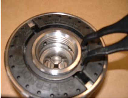
Showing circlip snapped closed
