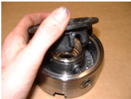
Lining up backing plate with pinions
