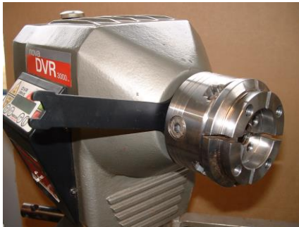
Using 11/2" Spanner to remover chuck from lathe
