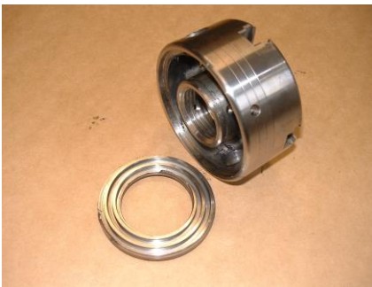
Removing scroll ring from Chuck
