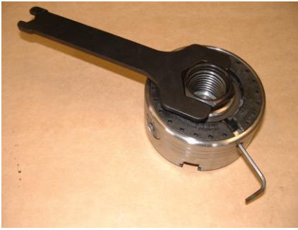
Using 1 1/2" spanner to re-attach insert.
