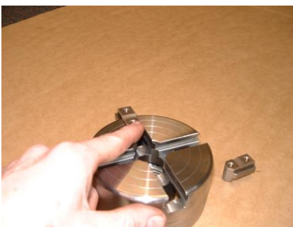
Removing jaw slides by hand
