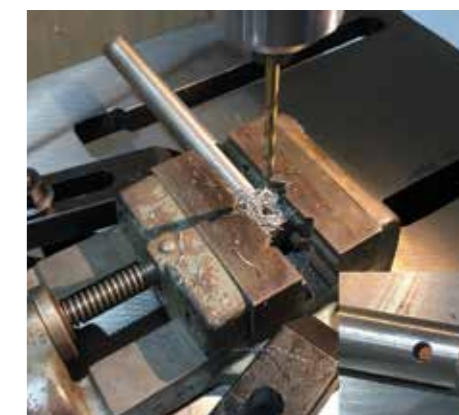
This shows my machine vice holding the round bar. The vice is secured on the table using parts from a universal clamping set. The inset shows the completed hole
