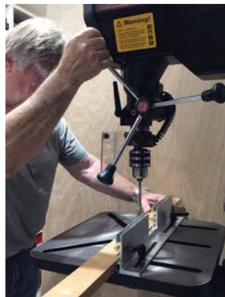
I am using a 25mm spade bit to drill a beech test piece. The setup sequence shows selecting the drill bit type, size, material being drilled and confirming that speed. I then set the self-start option, which is only two clicks
