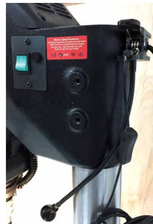
The lack of a work light is easily fixed courtesy of IKEA and about £6!
