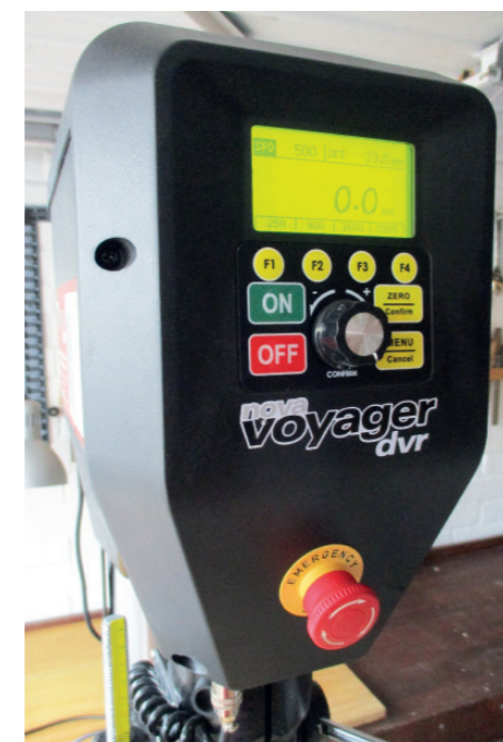
The control panel and lockable stop switch
