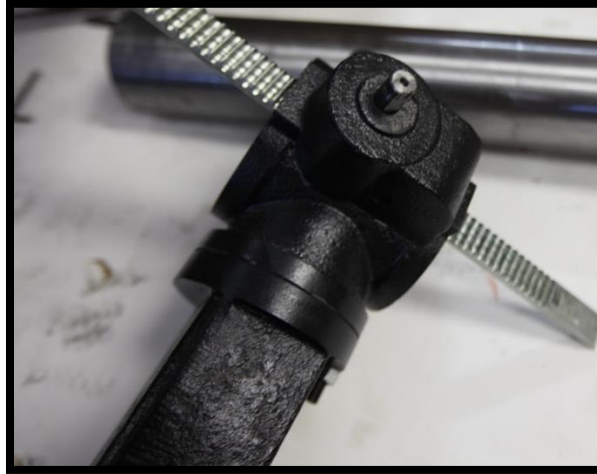
Figure 3 - Mounting the table bracket and rack 1/2
